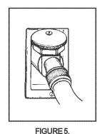
5 Disconnect the vent pipe from the draft hood where it connects to the water heater. In most installations the vent pipe can be lifted off after any screw or other attached devices are removed. Dispose of the draft hood. The new water heater has a draft hood which must be used for proper operation.
